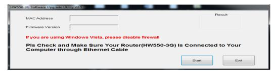
6. Connect your PC to any of the available Ethernet LAN ports of your HW550-3G using an Ethernet cable then click **Start**.
